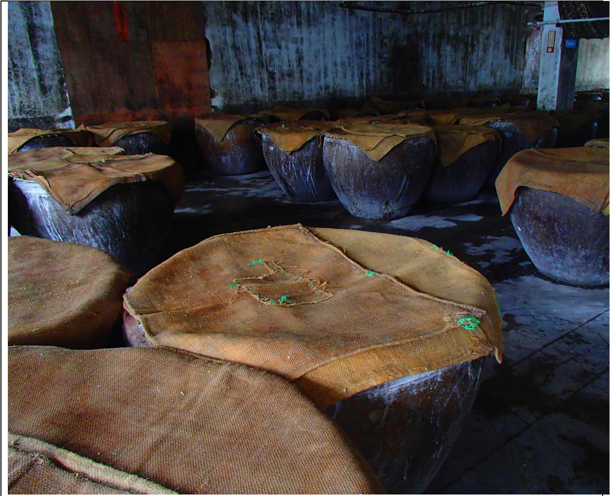
The gangs are covered with hemp cloth, and stored at a temperature of between 30 to 35°C for about 30 hours. The resulting product after the initial fermentation is jiuniang 酒娘.
