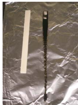
Before and after picture of a failed UL94 test. The specimen on the right failed because it dripped and did not self-extinguish quickly enough.
