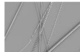
Figure 1 3000x magnification of 35%wt P4VP fibers
