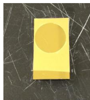
Figure 1. Teflon tape revealing 12mm diameter hole for imprinting
