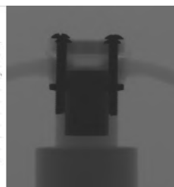
Figure 4: X-ray image of flow chamber
