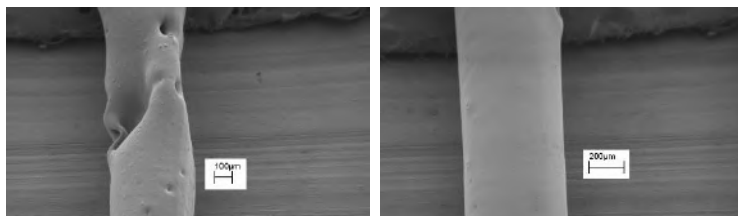
Figure 3. Comparison between SEM images of PLA with 10% graphene extruded 2500 mm/min at 185 °C (left) and at 230 °C (right). (Magnification: 150x)
