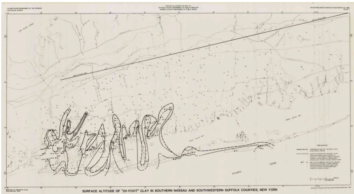
Figure 3 – Doriski & Wilde-Katz (1983) maps the presence and surface contours of the 20-Foot Clay in Nassau and Suffolk counties in Long Island. The 20-Foot Clay is an interglacial or interstadial marine clay within the Upper Glacial Aquifer. It is likely the same stratum as Fuller’s Vineyard Formation.
