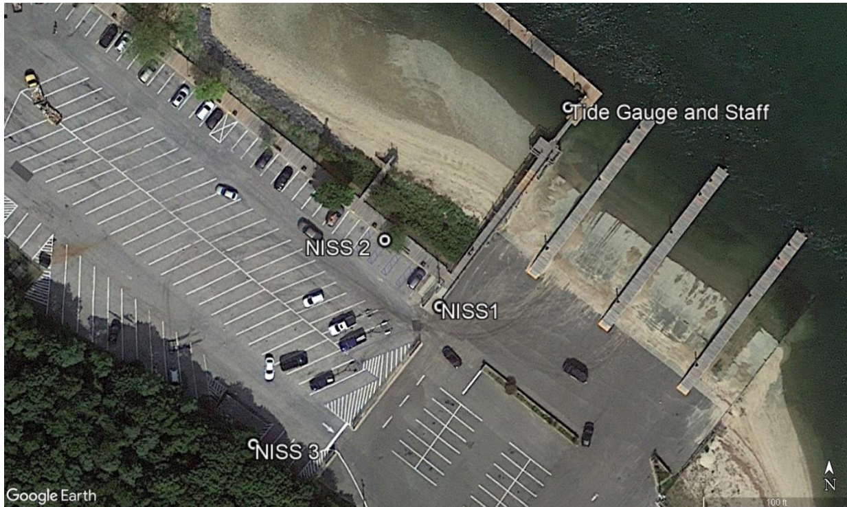
Figure 4 Locations of the three benchmarks and the tide gauge at the mouth of the Nissequogue River.
