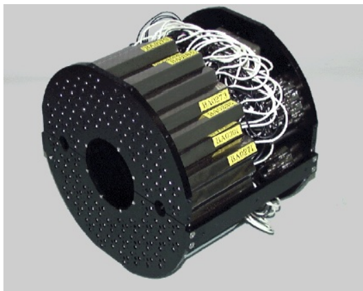
Figure 2.6: Photograph of one BBC barrel before the installation.
